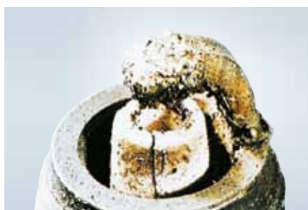
Melted center electrode
