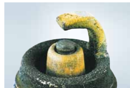
Severe center-electrode wear
