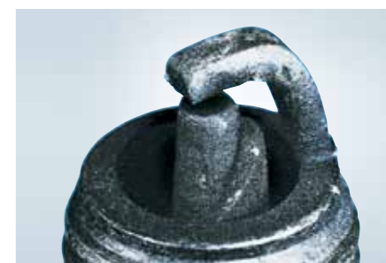
Cracking of insulator nose
