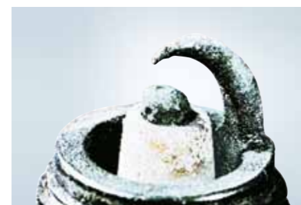
Severe ground-electrode wear
