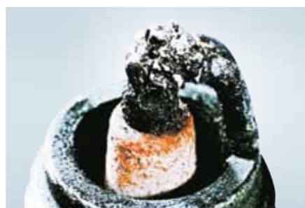
Partially melted electrodes
