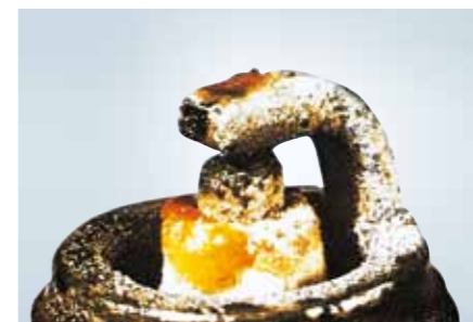
Severe lead deposits
