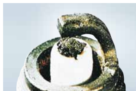
Partially melted center electrode
